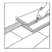
10.To lay the last row: position a loose board exactly on top of the last row laid. Place another board on top, with the tongue side touching the wall. Draw a line along the edge of this boards, to mark the first board. Cut along the edge of this board to mark the first board. Cut along this line to obtain of the required width. Insert this cut board against the wall. The last row
