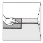
4.At the end of the first row, leave an expansion gap of 1/4" to the wall and measure the length of the last plank to
