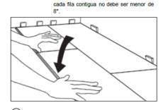
8 Angle up and push forwards until the boards lock together. Install the next planks as per picture No 6.
