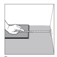
At the end of the first row, leave an expansion gap of 1/4" to the wall and measure the length of the last plank to fit.
