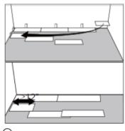
4 To cut the plank, use a simple utility knife and ruler, and with the top side facing up, cut heavily and several times on the same axis. The knife will not go through the surface but make a deep cut. You can then lift one half of the plank using your other hand to hold down the second placing it very close to the cut. The plank will split naturally.
