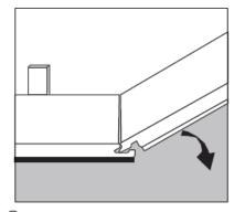
Insert the end section of the next floorboard at an angle to the first one, then lay down. Complete the first row in the same manner.
