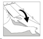
6 Lock the short end of the floorboard by inserting the tongue into the groove at an angle and dropping it into place. IMPORTANT: Make sure it is tightly locked with no gap.Then slide the floorboard towards the previously installed row until the tongue just touches the groove.
