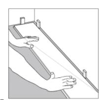
The subfloor should be level within 3/16" over 8 lineal feet, After thoroughly cleaning the subfloor, you should begin laying from left to right. Place the floorboard 1/4" from the left wall. Use spacers between the wall and the floorboard.
